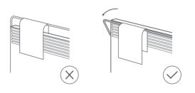
Note: Place the heater on level ground and do not hang a load of more than 1.5 kg on the drying rack.
