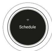
Note: The scheduled time here is the scheduled completion time, for example six hours, which means cooking will be completed in six hours, and the scheduled time cannot be shorter than the cooking time.
