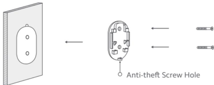
6. Keep the button of the outdoor camera facing downwards and rotate the base of the outdoor camera 180° so that the anti-theft screw hole faces downwards.
